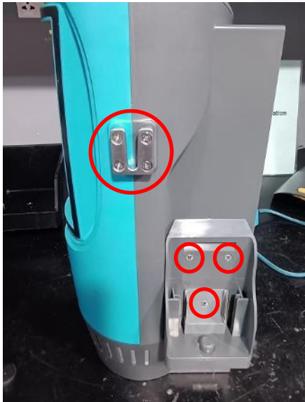
M4*10 FLAT HEAD SELF-TAPPING SCREW 106.1111.28 (6x)
